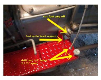
First you will need to cut off the foot peg. It is in the way of where the new linkage will be moved to. My floor board had a brace that hung off the foot peg for added support; I had to cut it off. I used that steel to beef up the brace that bolts to the tractor. Next you will need to drill two ½" holes for the throttle linkage to pass through. They don't have to be perfect but you do need to remove any burrs that could cause it to bind. 1" in from the edge and 2 ½" apart.
