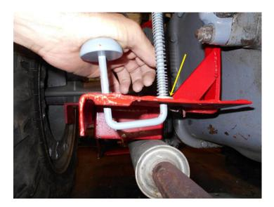
And for the finished product we now have a foot feed that is built into the running board.
