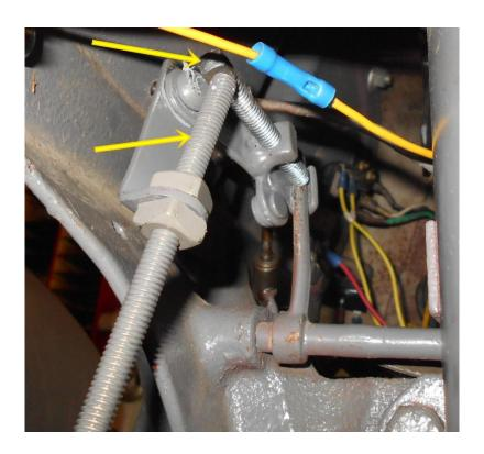
My kit was missing the bolt, instead of waiting for them to send me one I just made one. You will need to use 5/16" x 18tpi threaded rod and a coupler to extend the Dowden linkage because the foot feed is mounted lower and therefore is father away. The threaded rod in this
